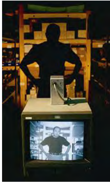
Figure 12: Active infrared night vision [47].
