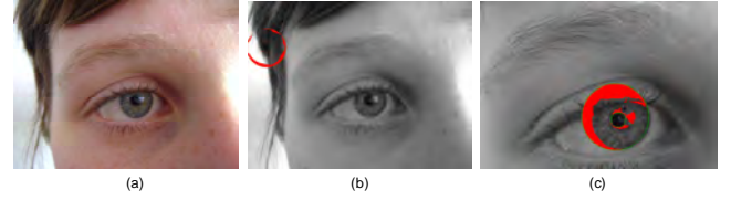
Fig. 3. Necessity for ROI extraction; (a) Captured eye image; (b) False iris segmentation; (c) Accurate iris segmentation with ROI image.
