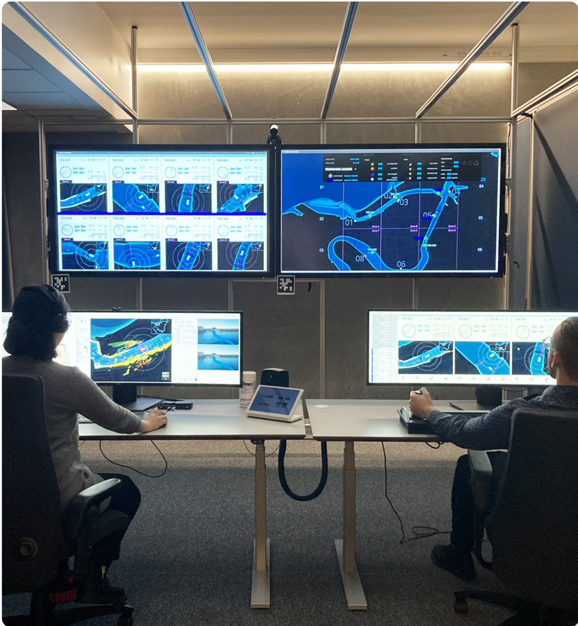
The control room at the NTNU Shore Control Lab where two operators monitor an autonomous ferry operation with multiple vessels. Photo: Jooyoung Park/NTNU
