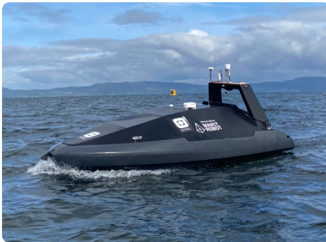
Figure 1 The Grethe ASV used for field trials in the spring of 2023. The trials were used to test the effect of using risk information for decision-making under real operating conditions.
