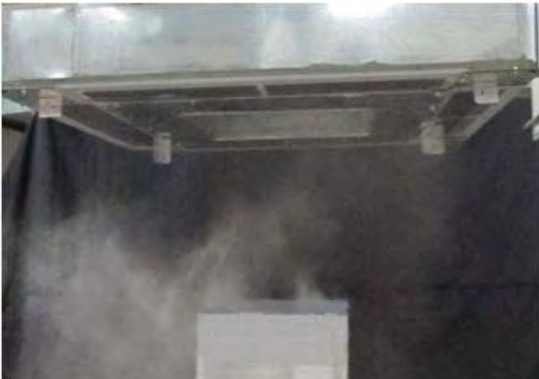
The air curtain is not formed
