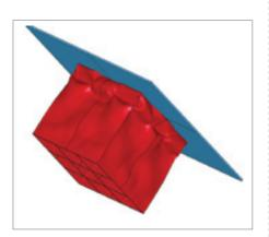
Figure 18 – Crash box during deformation in a numerical simulation involving the new constitutive model.
