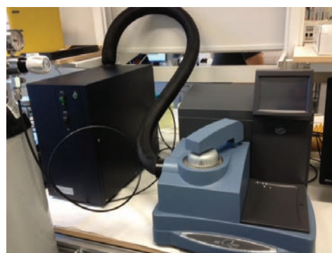
Name: TA Instruments Q2000 Differential Scanning Calorimeter
