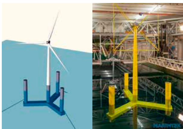
Figure 31: The 5-MW braceless semi-submersible wind turbine concept (left) and the 1:30 scale model tested at MARINTEK using hybrid testing techniques.
