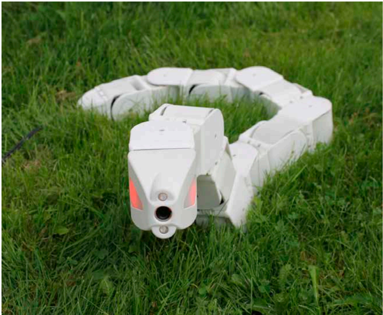
Figure 48: Mamba – a novel snake robot prototype.
