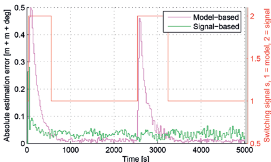
Figure 23: Estimation error of the signal-based and model-based observer parts, and the switching signal indicating which estimates are used in the closed loop.
