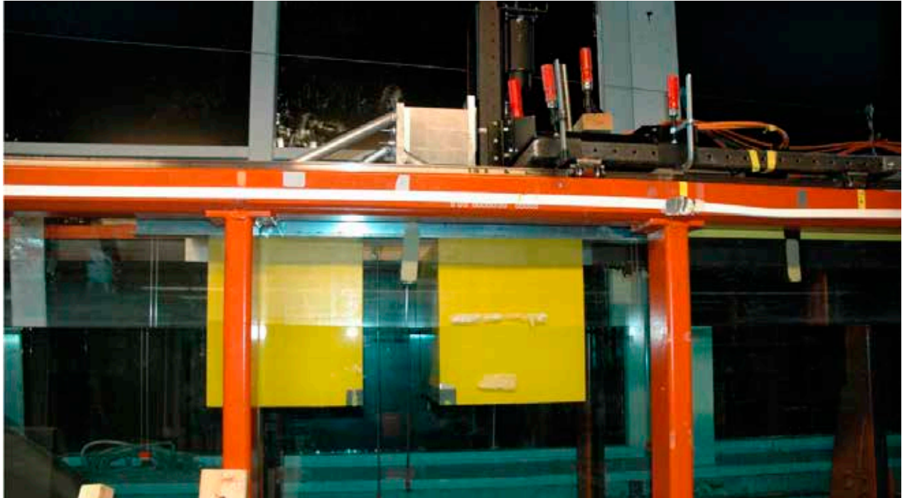
Figure 13: Experimental setup for 2D moonpool studies.
