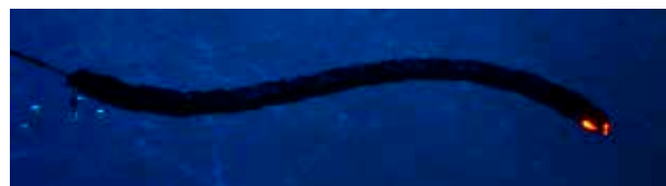
Figure 2: The underwater snake robot Mamba developed at NTNU to support the research on both ground and underwater snake robot locomotion. Markers are attached to the tail of the robot for position measurements.
