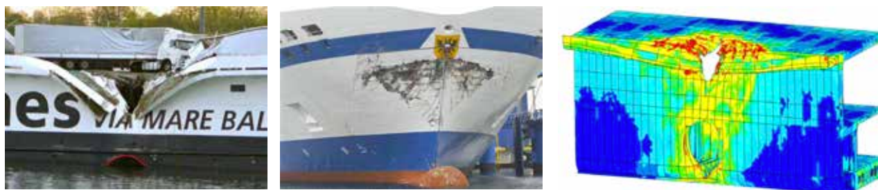
Figure 19: Actual damage and simulated damage.
