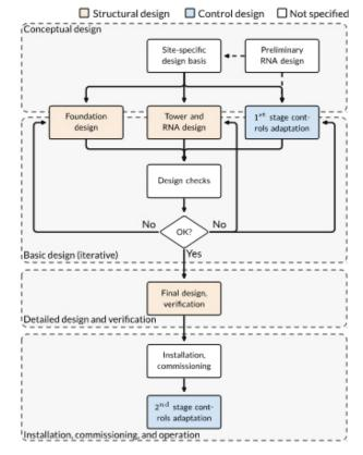
**Figure 19:** Outline of the design process for an offshore wind turbine with a two-stage adaptation of load reducing controls (Based on information from Seidel et al., Fischer et al. and IEC 61400-3)
