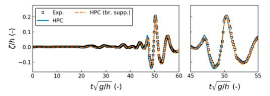
**Figure 7:** Non-dimensional wave-elevation time series for a focused wave in shallow water.  $\zeta$ , h, t and g are wave elevation, water depth, and time and acceleration of gravity, respectively. Exp.= experiments by Dommermuth et al. (1988); HPC and HPC (br. supp.) = HPC results without and with wave-breaking suppression, respectively.
