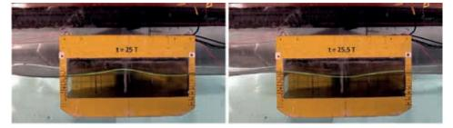
*Figure 2:* Second sloshing mode inside the damaged compartment in beam sea waves with period T
