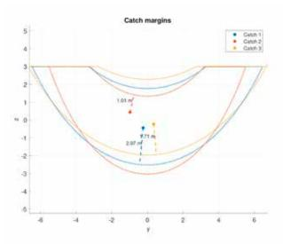
**Figure 3:** Margins for missing the catch for each of the three catches. The smallest margin and direction are marked.
