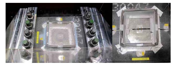
*Figure 15:* Left: Plate with initial crack in the middle subjected to cooling from liquid Nitrogen. Right: Brittle crack propagated from the middle crack and stopped closed to plate edges with higher temperatures.
