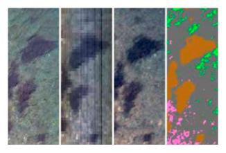
**Figure 11:** Airborne payload data. From left to right, first an image captured by the high resolution RGB camera, then an RGB representation of the hyperspectral data of the same region. On the third panel, an RGB representation of the same hyperspectral data after enhancement through fusion with the high resolution RGB image. Finally, classification using the same classes as in the UHI images.
