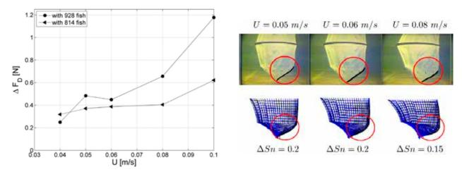
**Figure 3:** Fish farm in current. Left: Experimental relative drag change  $\Delta F_{D}/F_{D}$  caused by live fish. Right: Experimental (top) and numerical (bottom) net deformation in the experiment with 814 live fish. The area inside the red circle indicates the touching area.  $\Delta S_{n}$  represents the increase of solidity ratio at the back-cone part of the cage modeled in the calculations.
