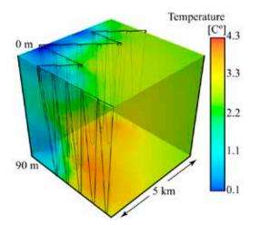
**Figure 3:** Path generated from measurements of the front. The cold water masses are shown as blue in the figure, and the black line illustrates the path of the robot.
