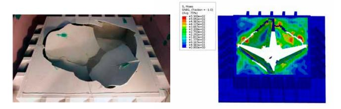
**Figure 14:** Left: Drop test carried at a temperature of -100°C. (Kim KJ, Lee JH, Park DK, Jung BG, Han X, Paik JK. An experimental and numerical study on non-linear impact responses of steel-plated structures in an Arctic environment. I.J of Impact Engineering. 2016;93:99-115). Right Numerical prediction of the deformation mode. The fringe plot shows the von Mises stress field (in MPa) at the end of the simulation.
