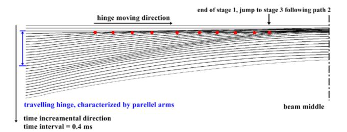
**Figure 18.** Snapshots of displacement profiles for a half plate strip during water entry; the plate thickness is 6 mm and the initial impact velocity is 10 m/s. The time interval is 0.4 ms. The red points denote positions of the traveling hinge at each time instant.
