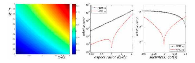
**Figure 6:** Local analysis for a cell with dimensions dx, dy, assuming a true velocity potential  $\varphi$  with contour plot in the left. Relative error as a function of cell aspect ratio dx/dy (middle) and of cell skewness cot  $\gamma$  (right) for a standard finite-difference method (FDM) with local 4th-order accuracy and for HPC. The latter allows local 8th-order accuracy.
