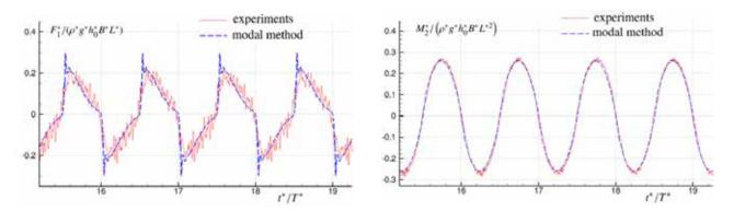
**Figure 4:** Evolution of global force (left) and moment (right) for  $\vartheta_0 = 4^\circ$ ,  $\sigma/\sigma_r = 1.0027$ .  $\vartheta^0$  and  $\sigma = 2\pi/T$  are roll excitation amplitude and frequency, respectively.  $\sigma_r$  is the first linear resonant frequency.  $L_{\sigma}$  B and  $h_0$  are the tank length, the tank width and the filling depth, respectively. Variables with symbol \* are made non-dimensional.
