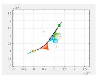
**Figure 5:** The optimal path from the starting location (yellow) to the final location (green). The red crosses mark possible emergency landing sites. It is indicated which emergency landing site should be chosen at each point along the optimal path.
