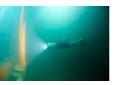
*Figure 1:* The Eelume articulated intervention-AUV inspecting a subsea installation (Courtesy: Eelume)
