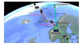
**Figure 1:** HYPSO Concept of Operations (CONOPS). The goal is to enable quick communication among agents, imaging small target areas, automated on-board processing and the rapid downlink of images and other data products with relevant features for post-analysis and dissemination at NTNU mission control. calibrated data, high resolution, geo-referenced coordinates, target detection and a high signal-to-noise ratio.
