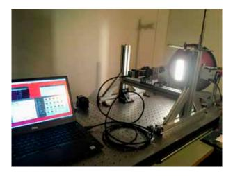
*Figure 6:.* Radiometric calibration of the HSIv6 with an integrating sphere
