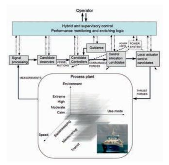
**Figure 12:** Block diagram of a hybrid control system for a marine vessel in an unknown environment.
