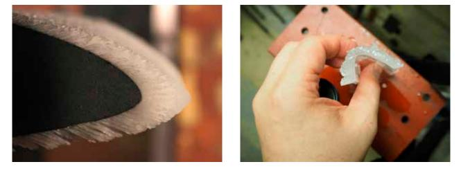
Figure 4: Examples of icing that was built up on the leading edge of wing during tests
