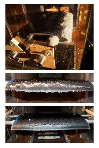
*Figure 5:* The upper and lower part show different kinds of icing accretion test during severe icing conditions.
