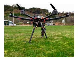
*Figure 7:* The HSIv6 mounted on the DJI S1000 octocopter UAV, from NTNU UAVlab
