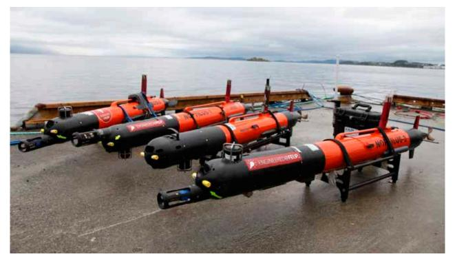
Figure 2: The AUVs used for the demo in the SWARMS project in the Trondheimfjord
