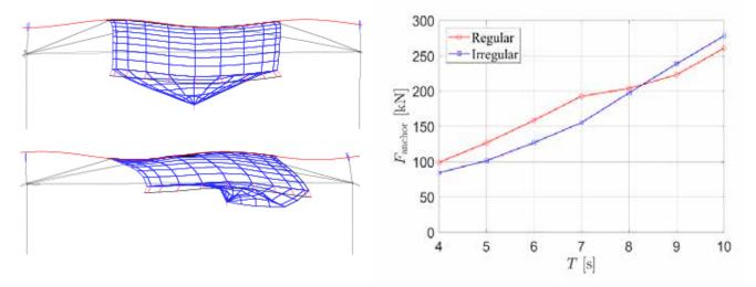
**Figure 2:** Left: Numerical net-based fish farm in regular waves (period T = 6, height H = 2.5 m), without current (top) and with current speed  $U_{\infty} = 0.5$  m/s (bottom). Right: Comparison of the maximum anchor loads by numerical calculations in irregular waves and equivalent regular waves. The considered regular wave steepness is  $H_{\lambda} = 1/15$ , the current velocity is  $U_{\infty} = 0.7$  m/s. The significant wave heights for irregular waves are given as  $H_{S} = H/1.9$ .
