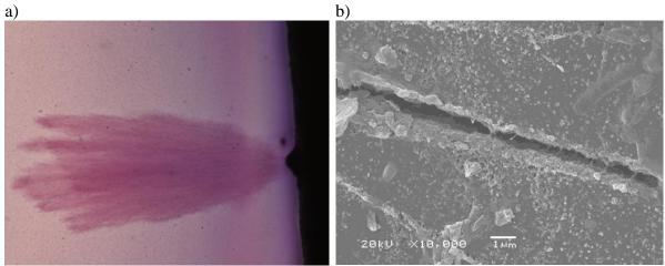
a) Vented water tree growing from the conductor screen in a 12 kV XLPE cable. b) SEM micrographs showing the surface of a conductor screen that has been in contact with a corroded section of the surface of an aluminium conductor strand.
