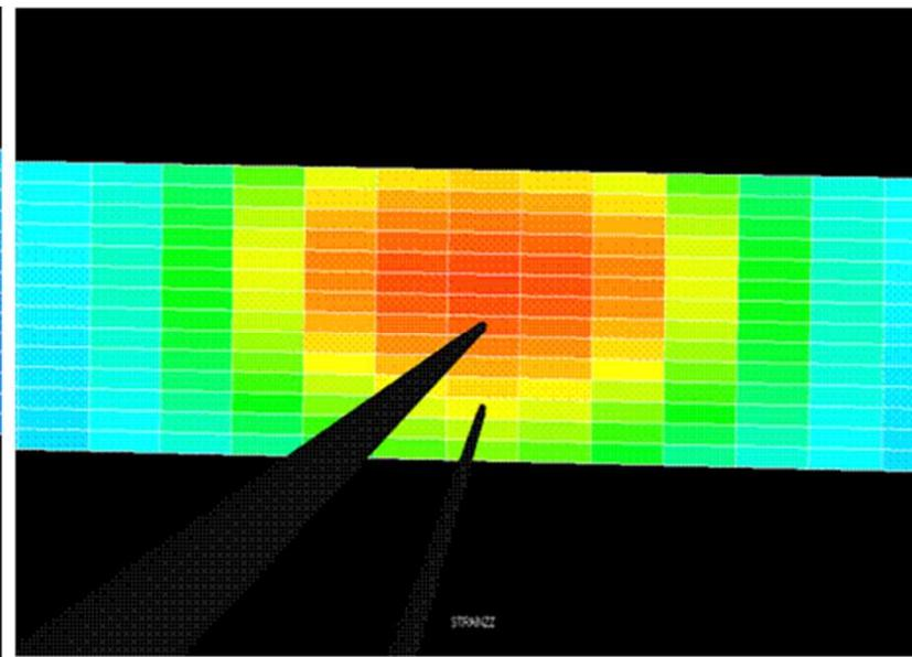
2. Injector Well - Strain Analysis – 0.062 in/in - 450 tons/day
