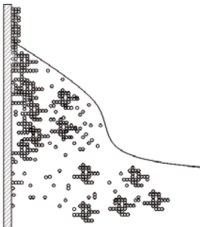
Figure 1. Illustration of thin-film formation by dip-coating from a sol of nanoparticles.
