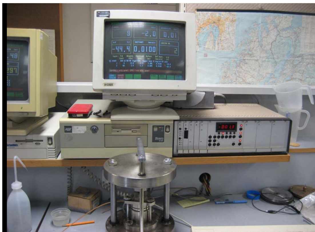
Fig. 6: Continuous loading Oedometer test on stabilized quick clay and laterite soils (CRS)
