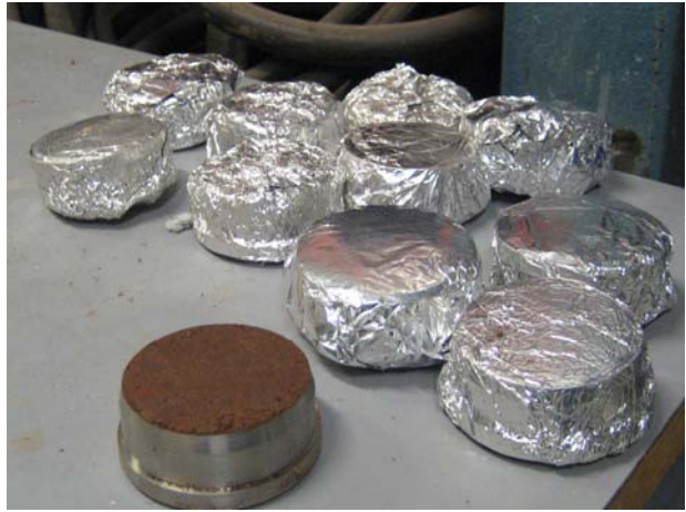
Fig. 4: Laterite samples prepared for oedometer test
