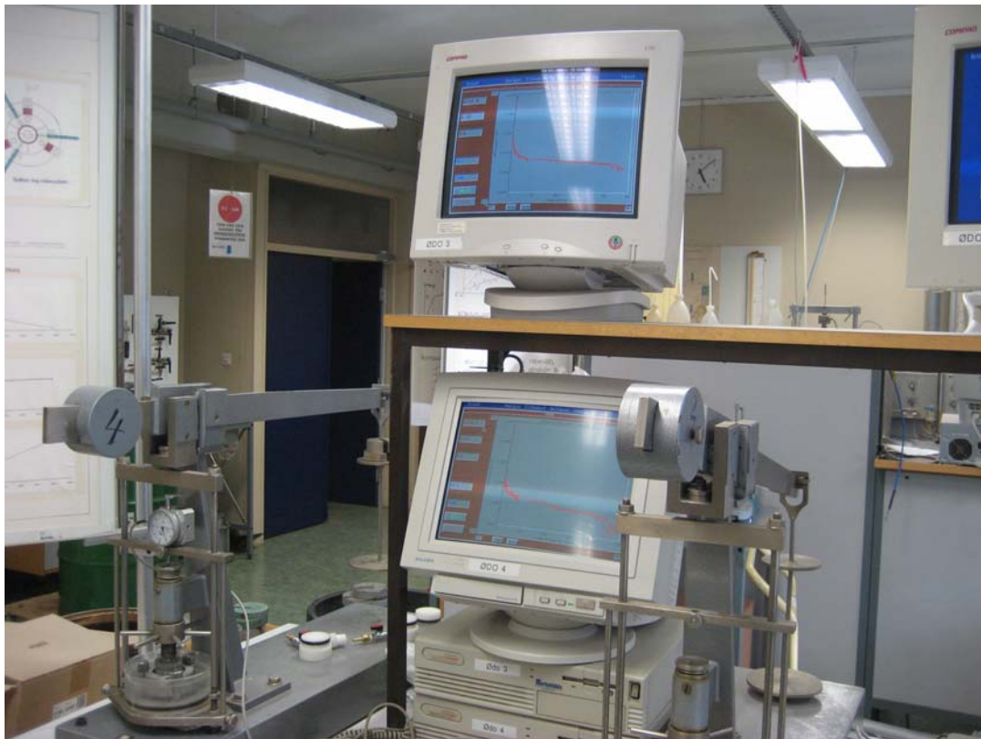
Fig. 5: Incremental load Oedometer test on stabilized quick clay and laterite soils
