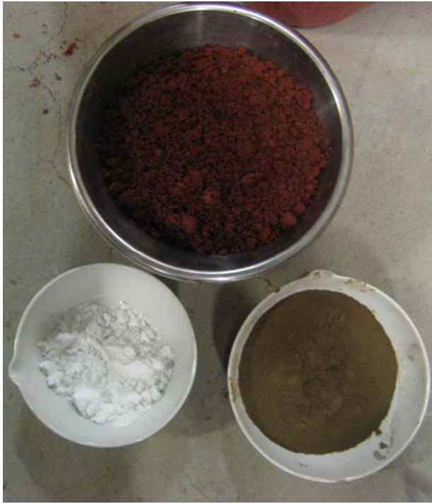
Fig. 3: Stabilization of laterite soil with lime and volcanic ash
