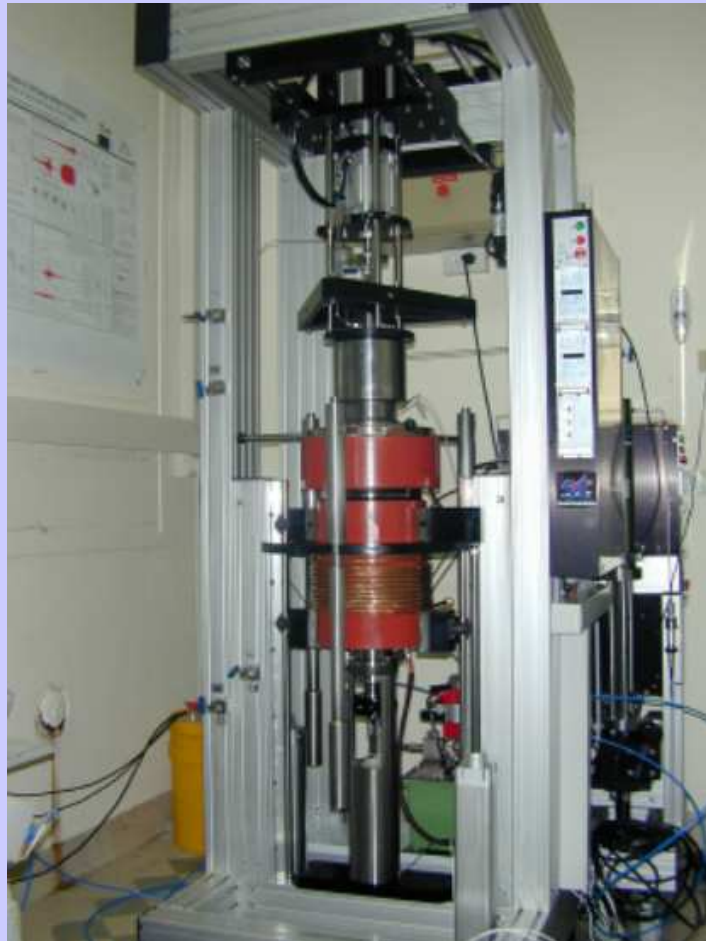
Triaxial apparatus at ENS, Paris
