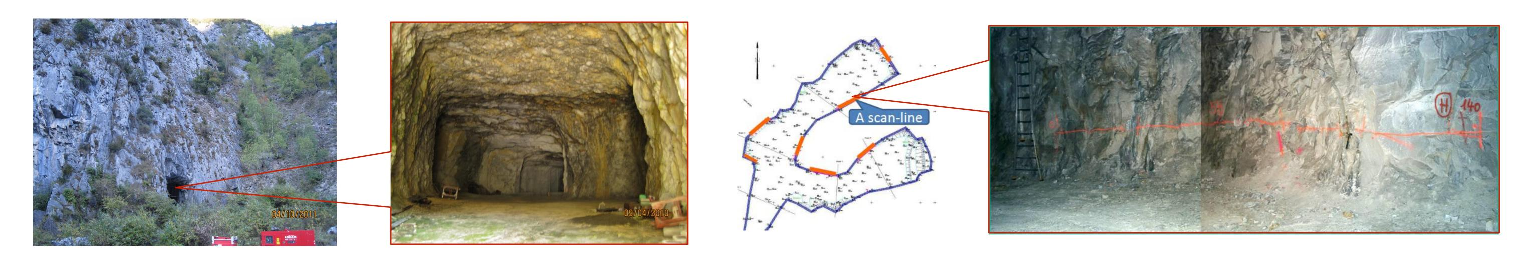
An alternative approach for fractured rock engineering has been proposed and applied for the first time in reality on the data of the castle gallery of Saint Béat.
