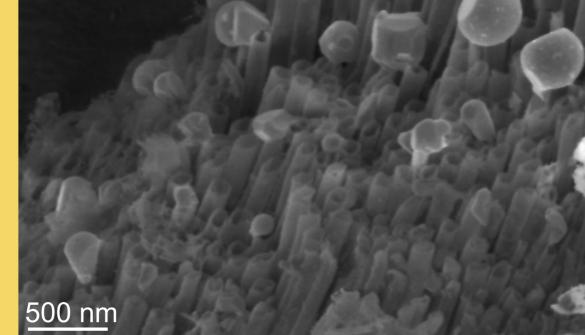
Al<sub>2</sub>O<sub>3</sub> Nanotubes, top view
