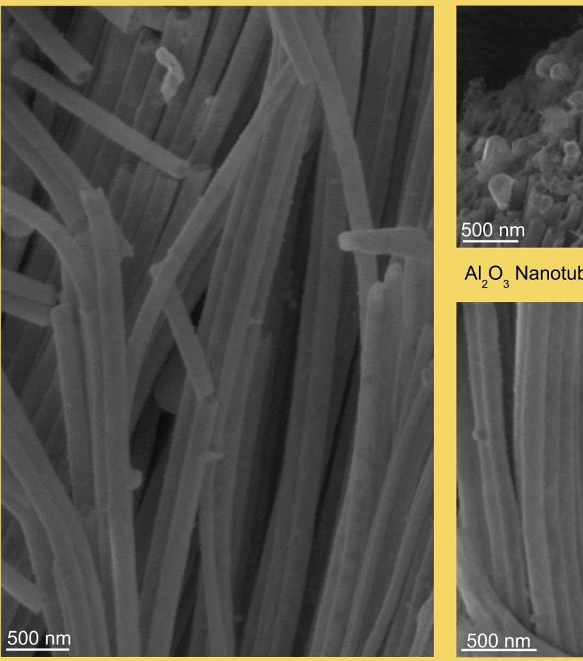
Al<sub>2</sub>O<sub>2</sub> Nanotubes, side view
