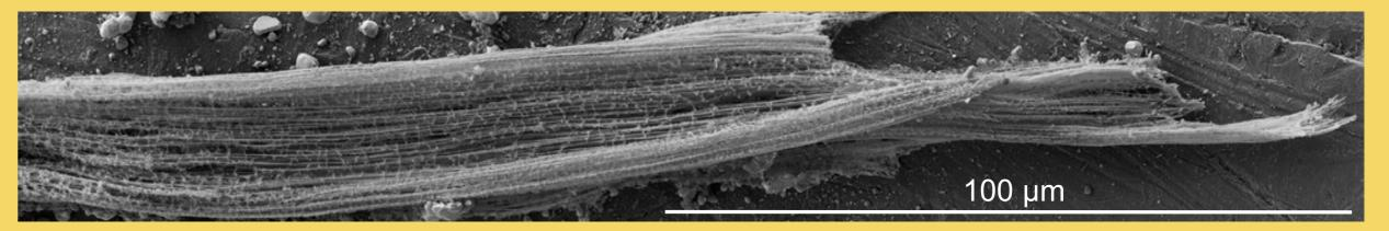
Cu Nanowires in a partially decomposed template
