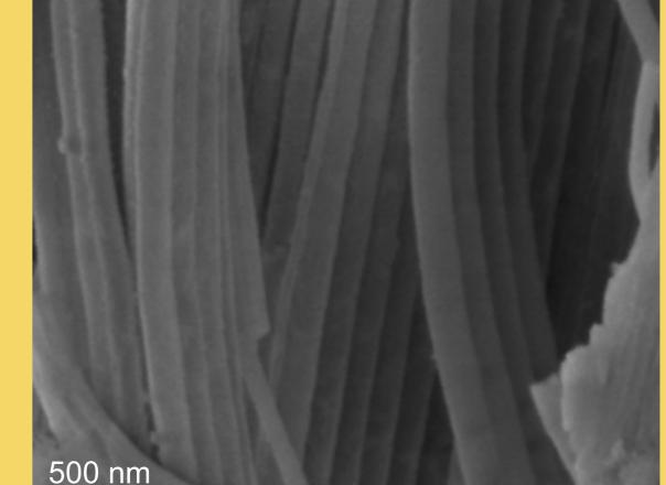
Al<sub>2</sub>O<sub>2</sub> Nanotubes, side view
