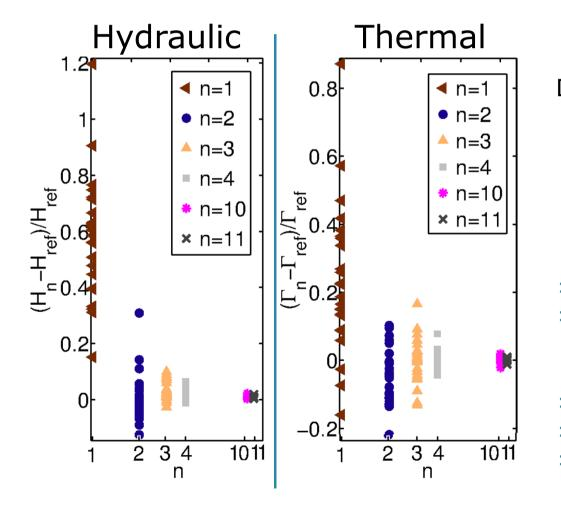
$(H_n - H_{ref})/H_{ref}$  and  $(\Gamma_n - \Gamma_{ref})/\Gamma_{ref}$ : Difference between the efficiencies in the filtered  $(H_n, \Gamma_n)$ and in the fully rough geometries  $(H_{ref}, \Gamma_{ref})$
