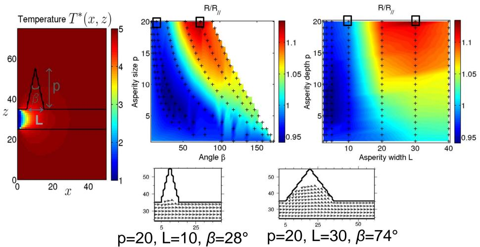
At small Pe: thermal exchange slighlty less good with the asperity
