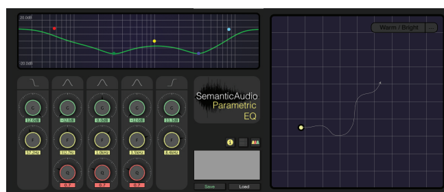
Figure 1: The extended Semantic Audio Equalisation plug-in with the two-dimensional interface. To modify the brightness/warmth of an audio signal, a point is positioned in two-dimensional space.
