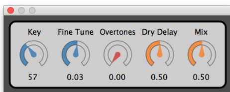
Figure 8: Audio plug-in for fixed f_R harmonizing effect. f_R parameter is labeled Key .
