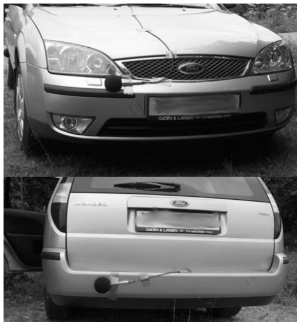
Figure 2: Example of microphone positions for direct vehicle sound measurements
