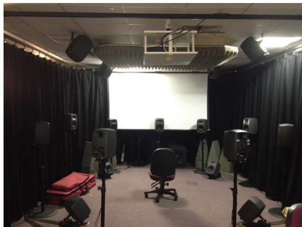
Figure 2: The listening room used throughout the experiment. Loudspeakers not part of the defined 7.1 playback system were non-active during the test.
