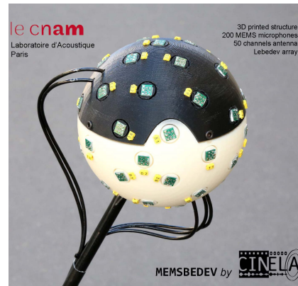
Figure 9: MemsBedev microphone arrays with N = 50 MEMS microphones
