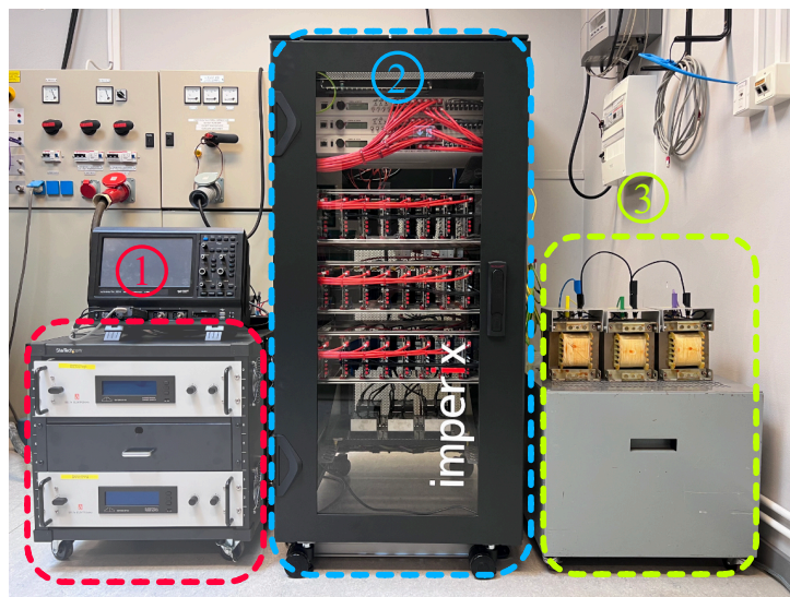
Fig. 18: Lab set-up of the MMC: 1) DC power supply 2) MMC 3) Three-phase RL load
