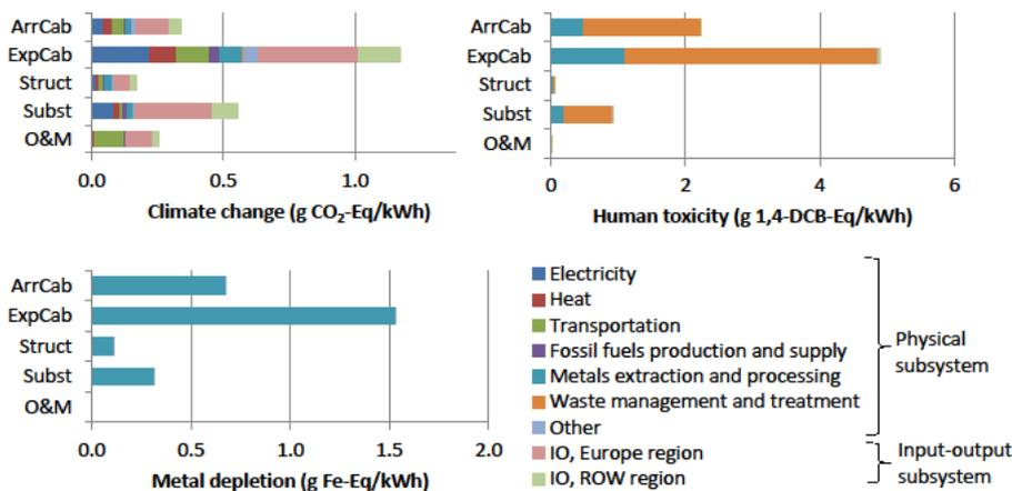
**Figure.** LCA results for a North Sea power grid by five components and nine stressor sources per kWh transmitted. Components: ArrCab = Array cables; ExpCab = Export cable; Struct = Substructure and topside for substation offshore; Subst = Electrical equipment (voltage source converter, transformer, breakers and switchgear) for substations offshore and onshore; O&M = Operations and maintenance. The reference provides results for seven additional impact categories.
