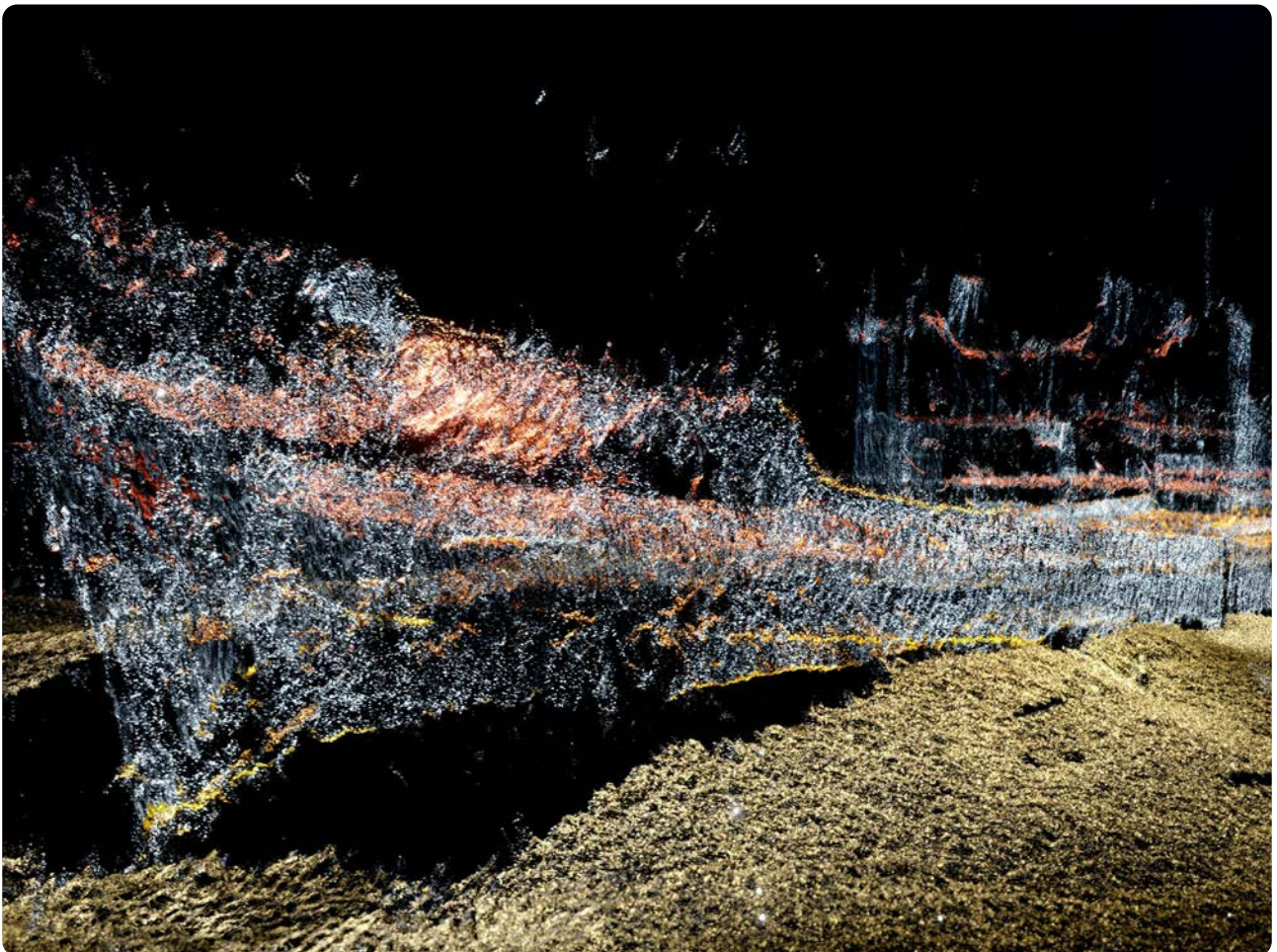
3D Render of SAS Bathymetry Showing a Shipwreck from a World War II Chemical Munitions Dumpsite in the Skagerrak Sea. Picture: Ole Jacob Lorentzen
