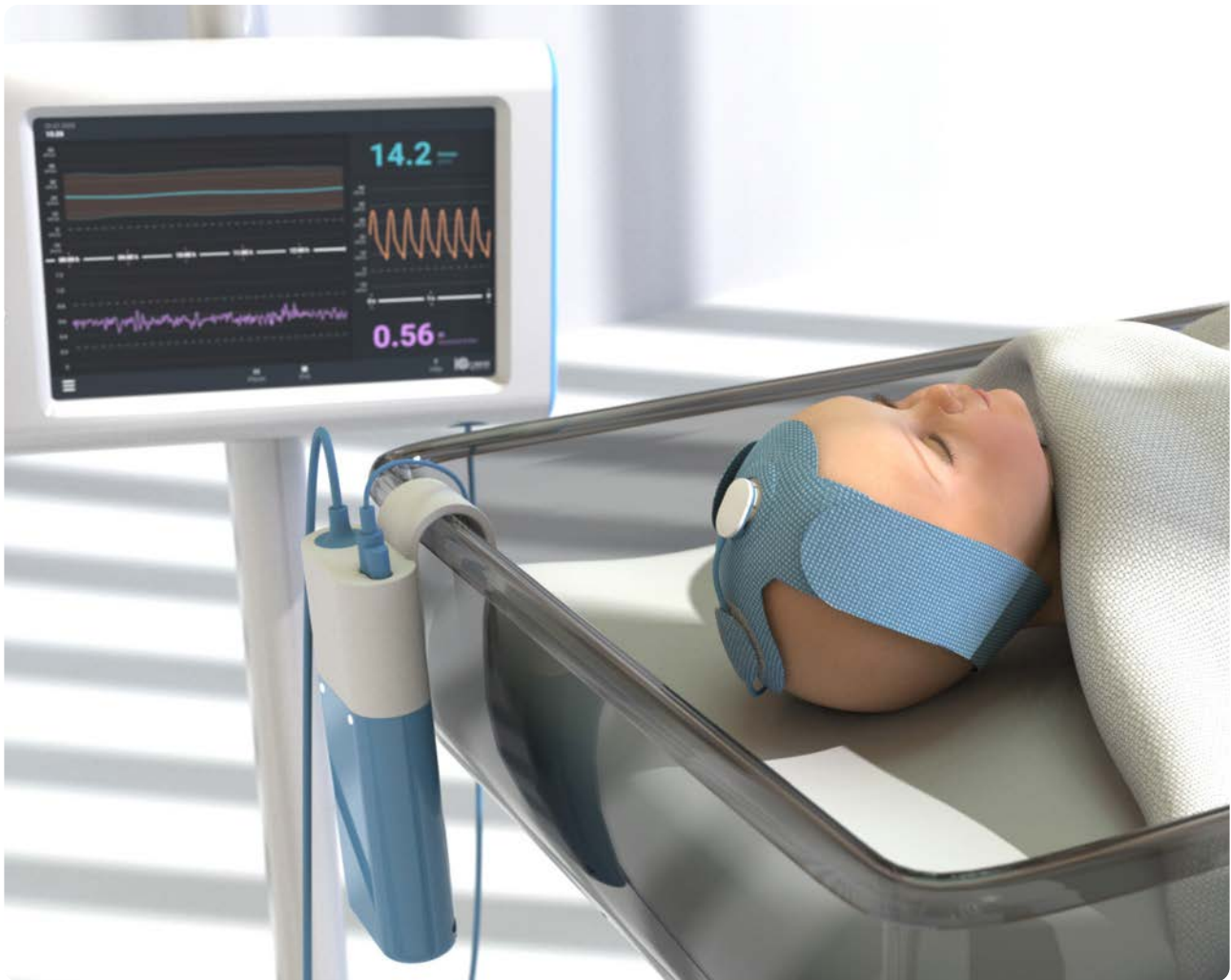
NeoDoppler: Professor Hans Torp at NTNU invented this technology. A tiny probe fastened to the child's head monitors brain perfusion over time.
