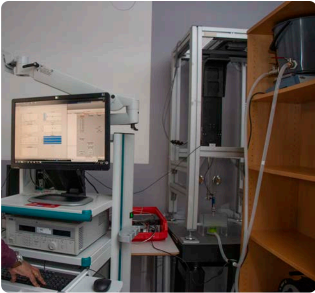
Experimental setup for estimating flow influx/efflux in oil and gas boreholes using pulse-wave Doppler ultrasound. Photo: Kari Williamson/NTNU
