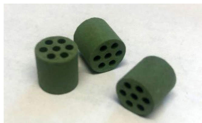
Figure 1. Fresh catalyst pellets of the type investigated in the study. Pellet length 1 inch.
