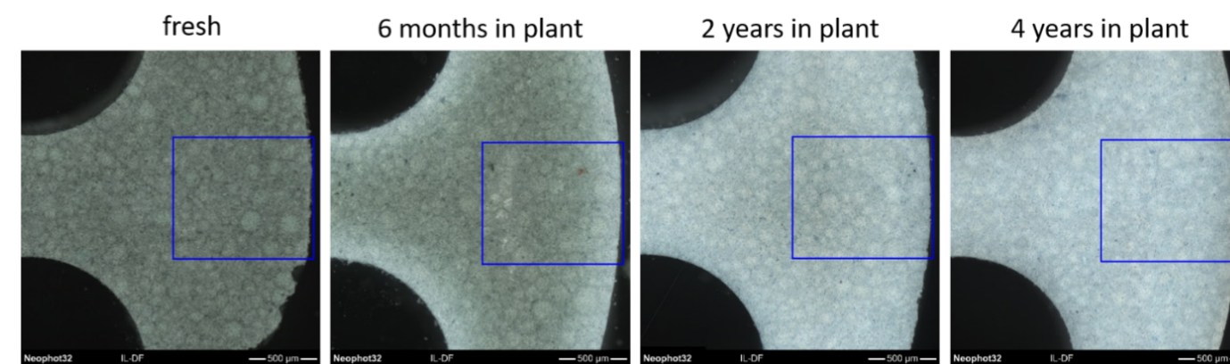
Figure 2. Light microscopy, dark field illumination image of polished cross-sections of catalyst pellets after varying times in plant
