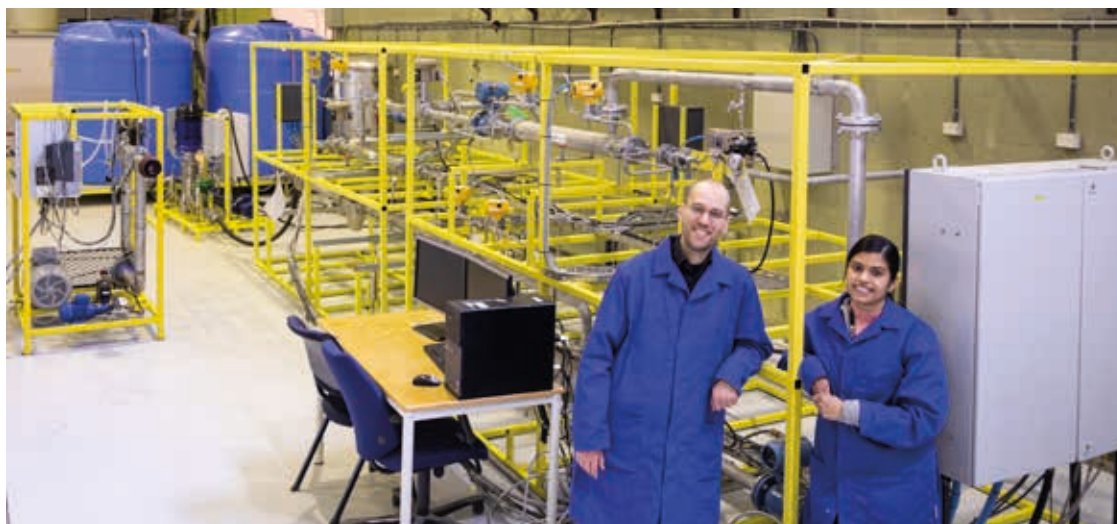
Hydrocyclone test rig with pump and tank system. PhD student Mishiga Vallabhan and her project manager and main supervisor Associate Professor Christian Holden
