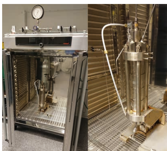
Figure: High pressure gas flotation cell: flotation cell inside the temperature-controlled cabinet (left) and the flotation cell (right). Attachment of an oil droplet to a gas bubble from a microfluidic experiments is shown below.
