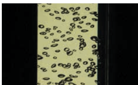
Figure 2: Image of gas bubbles in MQ water in the high-pressure gas flotation column.
