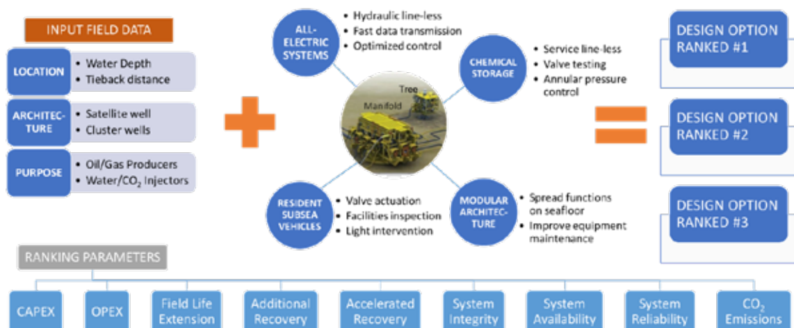
Figure 1. The combined concepts when applied to a subsea field may provide different design options for the production system. The research aims to identify the feasible solutions and rank them based on technical, operational, and environmental parameters.
