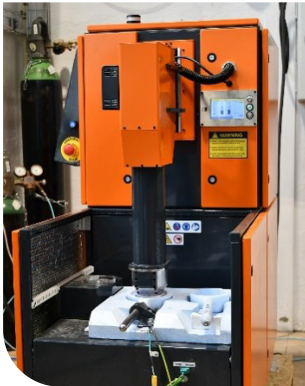
The Laser-induced breakdown spectroscopy (LIBS) used in the investigation of oxidation of molten aluminium.
