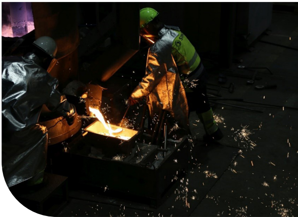
Pyrometallurgical processing of bauxite in the Pedersen process.
