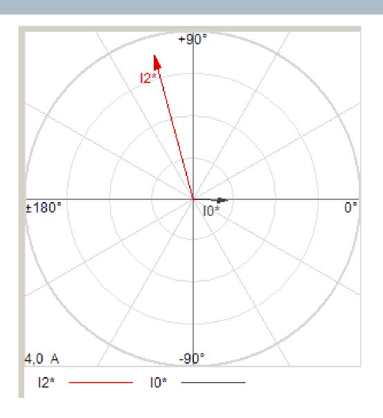
Analysing the **angle between I2 and I0** we can see that this criterion clearly identifies a **fault C-G or A-B**.
