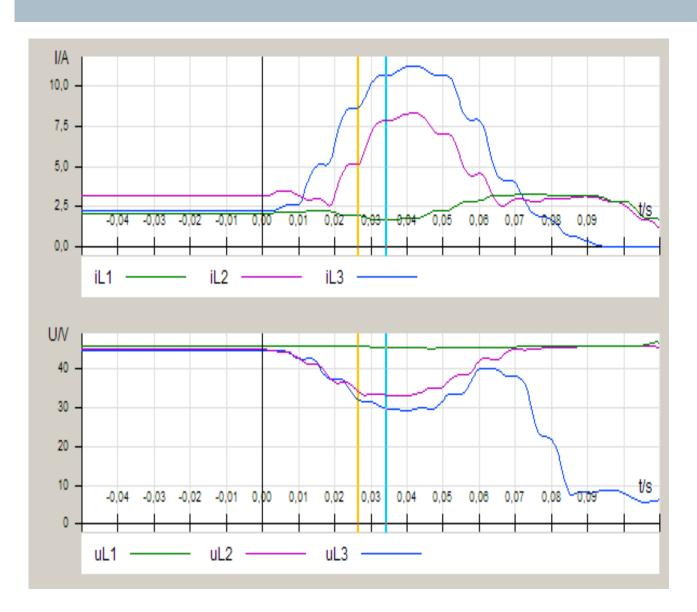
RMS of currents and voltages also give indication about the type of the fault
