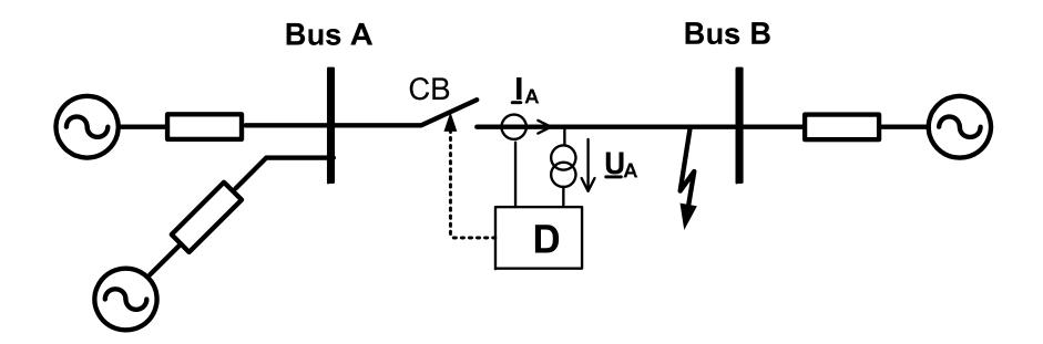
• Distance protection D determines the fault impedance  $\underline{Z}_F$  from the voltage  $\underline{U}_A$  and the current  $\underline{I}_A$  measured at the relay location according to Ohm's law:
