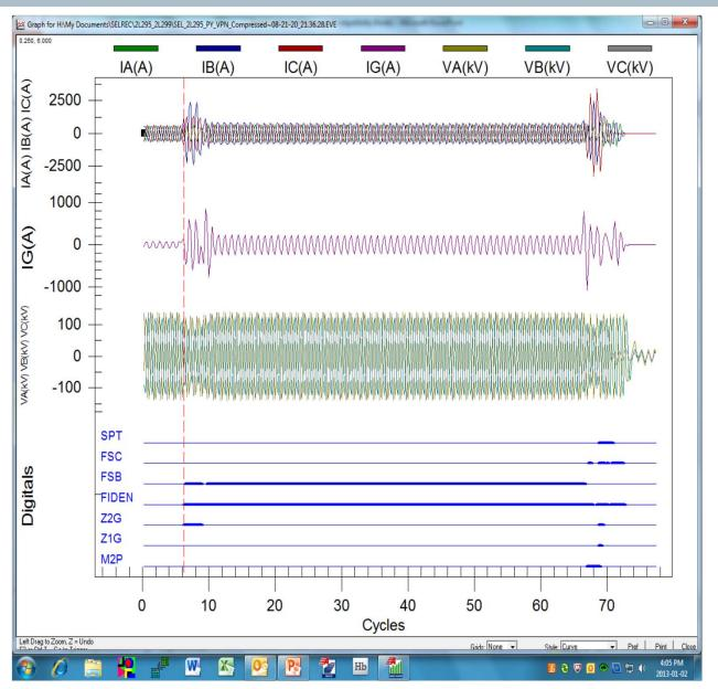
after reclosing to the B-C fault of line L1 at substation ABC the relay at XYZ selects phase C (see signal FSC)
