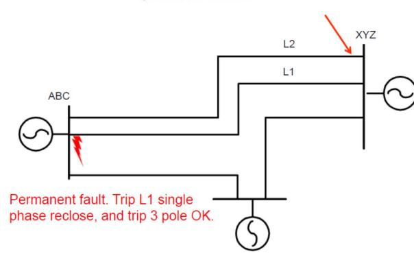
Substations ABC and XYZ are connected with parallel lines L1 and L2
