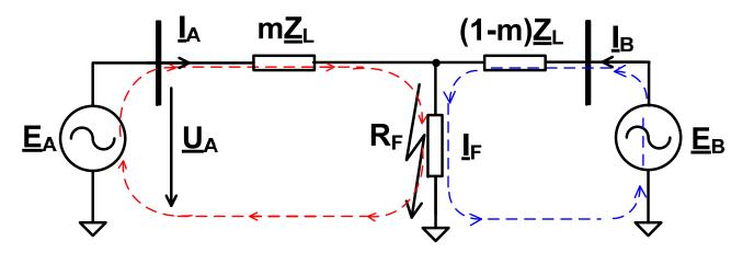
fault current from remote end causes additional voltage drop at fault resistance R<sub>F</sub>
