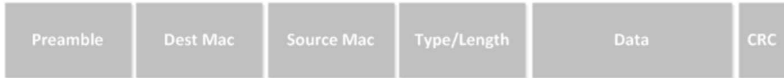
Original Ethernet Frame
