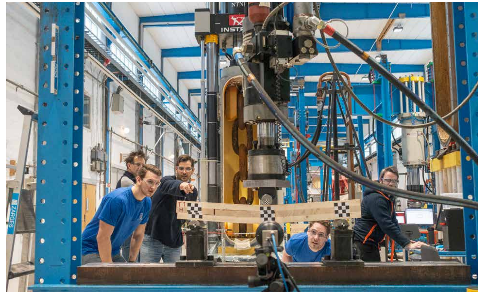
Master's in progress. Testing impact loading on beams of cross-laminated timber. From left: MSc student Lars Gruben, supervisor Professor Arild Holm Clausen, Associate Professor Haris Stamatopoulos (pointing), MSc student Sondre Skau Kentsrud, and Senior engineer Thomas Uhlving (Photo: Sølvi W. Normannsen).
