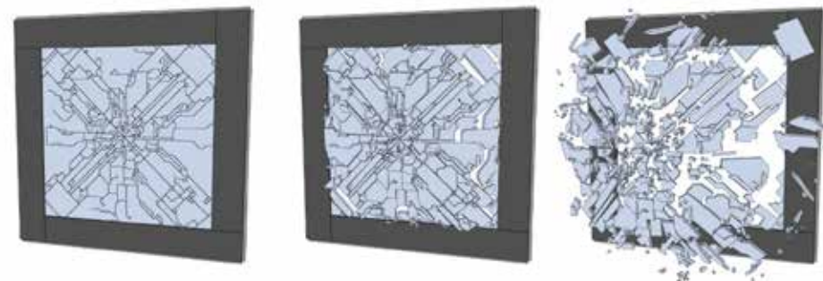
Comparison between high-speed camera images (top) and simulations (bottom) using the IMPETUS Afea Solver from a blast-load experiment in SIMLab's shock-tube on an annealed float glass.
