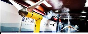
**The Ocean Basin Laboratory** has a depth of 10 metres and a water surface of 50x80m. It is excellent for investing existing or future challenges within marine structures and operations. A total environmental simulation including wind, waves and current offers a unique possibility for testing models in realistic conditions.
