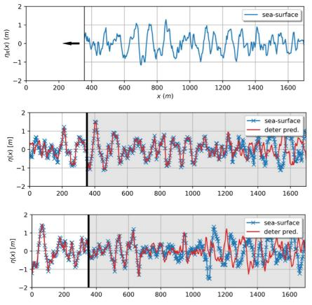
Figure 7. Forecasting of wave fields. Based on a "scan" of the sea surface (top), the wave field is predicted after 60 s (middle) and 120 s (bottom). The figures show both the predicted and the actual wave elevation.
