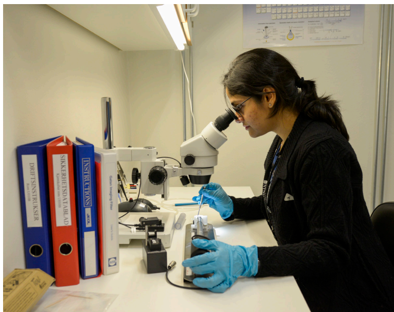
Postdoc Dipanwita Chatterjee inserting a specimen in the double tilt holder for 2100F.
