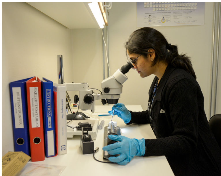
Postdoc Dipanwita Chatterjee inserting a specimen in a double tilt holder.
