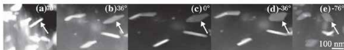
Figure 2. HAADF STEM tomography micrographs from tilt series at (a) 70°, (b) 36°, (c) 0°, (d) -36° and (e) -76° tilt angle. The arrow points to dispersoid 1 in Figure 1(b) and (c).
