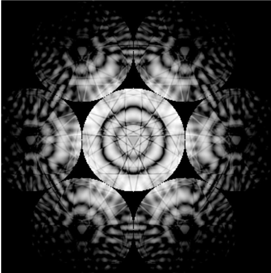
Simulated, 100kV, Si[111], 160 beams
