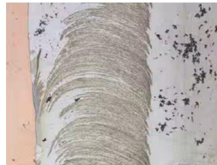
An optical image of a FSW copper- Aluminium Joint.
