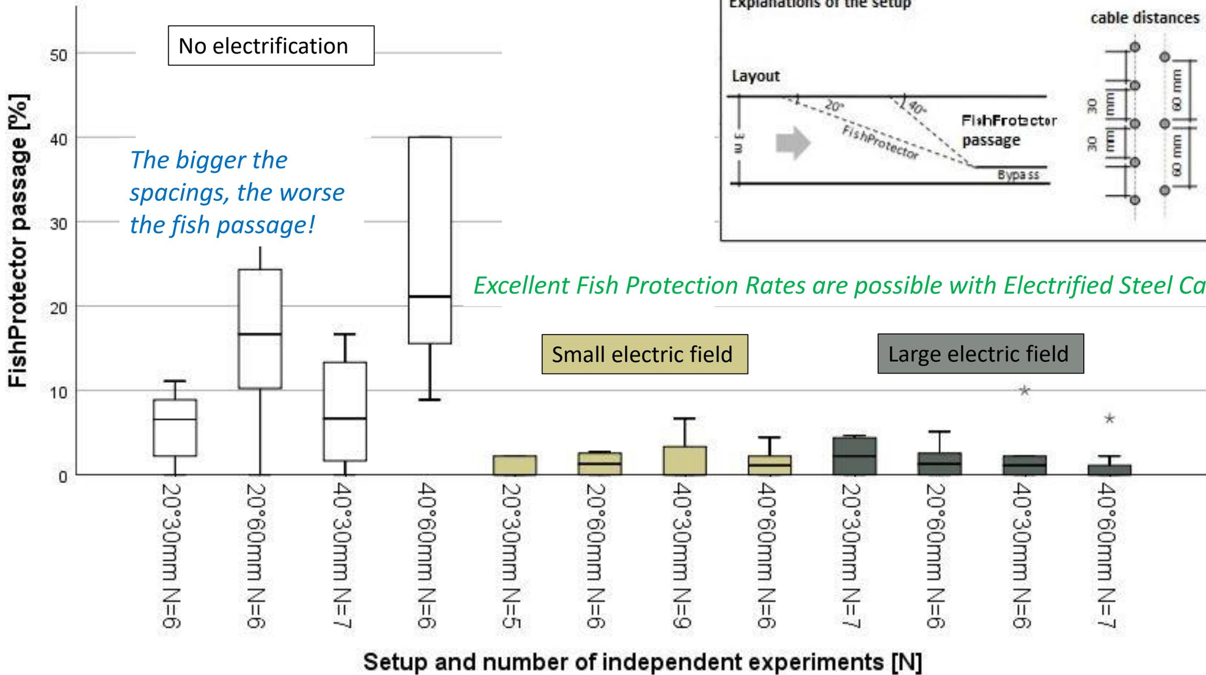
*Excellent Fish Protection Rates are possible with Electrified Steel Cables !!*
