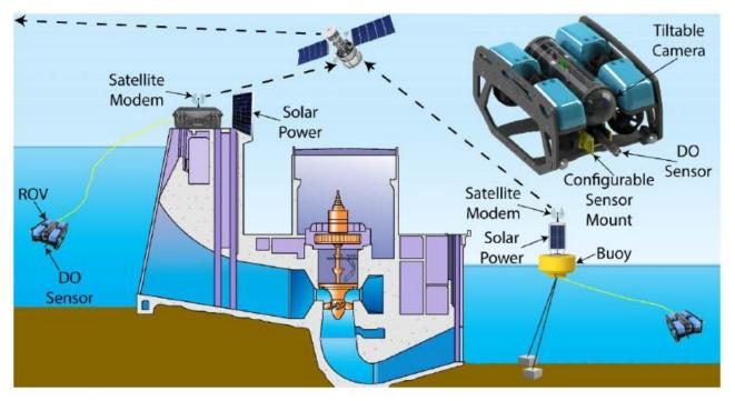
Figure 1. A visualization of the real-time and autonomous water quality monitoring system in operation.
