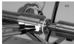
Figure 1: Setup of the dynamic punch test.
