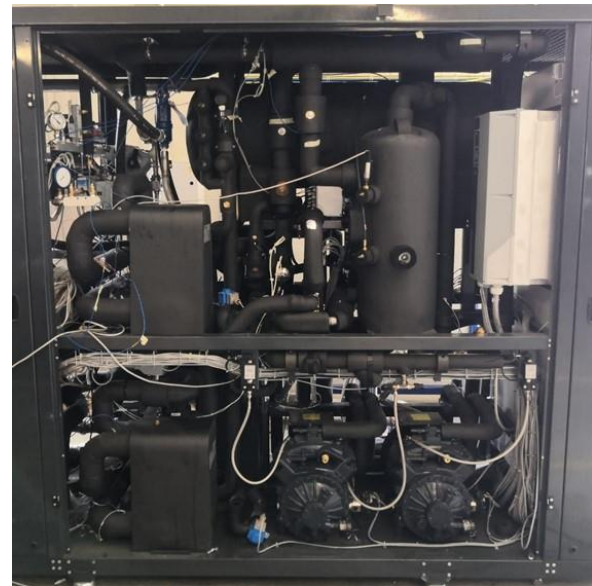
Figure 1: Transcritical heat pump (a) Schematic (b) Experimental apparatus
