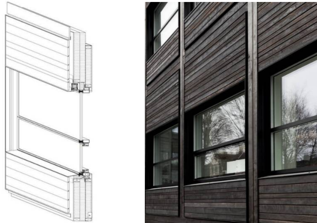
Figure 6.4 On the left schematic representation of the external wall having charred wood cladding as exterior layer and massive wood structure with a gypsum board on the internal side. The window is horizontally divided in two parts not equally high. On the right the external appearance of the building.
