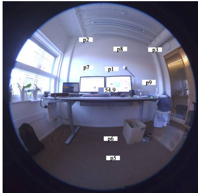
Figure 6.15 Fisheye image elaborated by Radiance to obtain luminance value in relevant points, values are reported in table 6.15.
