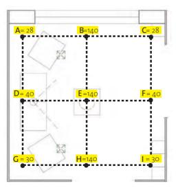
Figure 3.54: E values taken on the horizontal grid at a height of 80 cm from the floor level. I Artificial Lighting Solution.
