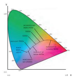
Figure 2.16 Chromaticity diagram for natural and artificial light sources.
