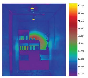
Figure 3.33: Second Artificial Light Solution. False colour image with luminance values.
