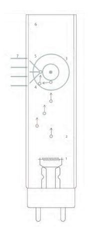
Figure 2.47: When leaving the electrode (1) the electrons (2) collide with mercury atoms (3). The mercury atoms (4) are thus excitedand in turn produce UV radiation (5). The UV radiation is transformed into visible light (7) in the fluorescent coating (6).
