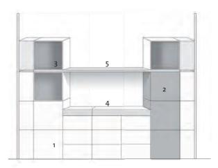
nels (150x55x3 cm. Figure 17. Component 4), one above the other, to create the work plane and one dark brown (250x30x3 cm. Figure 17. Component 5) which was used like a shelf to 1.50 meter high.
