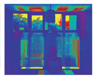
**Figure 3.43:** Second Natural Light Solution: sunny sky conditions. Daylight devices: Venetian Blinds and Light Shelf. Kitchen false colour image with luminance values.
