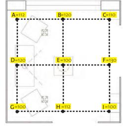
Figure 3.53: E values taken on the horizontal grid at a height of 80 cm from the floor level. I Artificial Lighting Solution.
