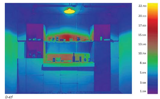
1° SOLUTION (Figures 3.46 and 3.47): The illumination appears scattered and uniform. The source creates in fact low shadows which tend to flatten the objects three-dimensions; at the same time the device itself, not being directed, causes negative shadows in some points like inside the right cabinet.
