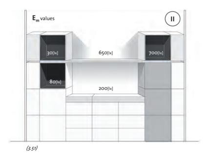
Figure 3.50 and 3.51: Em values are given by six E values measured on the horizontal grid in the cabinet planes and by three E values taken on the horizontal grids in the shelf planes. (See 7.2.4 Measurements)
