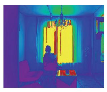
Figure 3.42: Second Natural Light Solution: sunny sky conditions. Daylight devices: Blinds. Living Room false colour image with luminance values.
