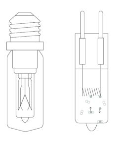
**Figure 2.45:** Halogen lamp for mains voltage with screw cap and outer envelope (left). The outer envelope means that the lamp can be operated without a protective glass covering. Low voltage halogen lamp without pin base and axial filament in a quartz glass bulb (right).
