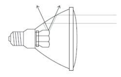
**Figure 2.46:** Lamp with dichroic cool-beam reflector. Visible light is reflected, infrared radiation trasmitted, thereby reducing the thermal load on the illuminated objects.
