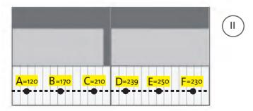
**Figure 3.31:** E values on the vertical grid at a distance of 8 cm from bookcase. II Artificial Lighting Solution.
