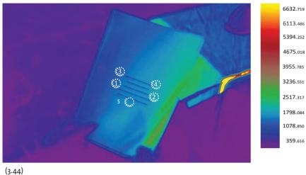
Zoom showing in detail luminance values on paper sheet (visual task plane). Figure 3.44: Second Natural Light Solution: sunny sky conditions. Daylight devices: Blinds.
