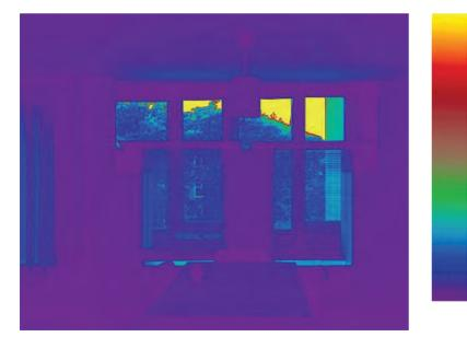
**Figure 3.41:** First Natural Light Solution: cloudy sky conditions. Daylight devices: Venetian Blinds and Light Shelf. Kitchen false colour image with luminance values.
