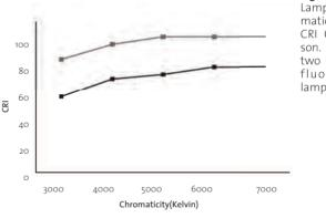
Figure 2.17 Lamp Chromaticity and CRI Comparison. Example: two different fluorescent lamps.
