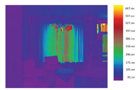
Figure 3.40: First Natural Light Solution: cloudy sky conditions. Daylight devices: Blinds. Living Room false colour image with luminance values.
