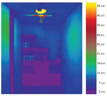
Figure 3.32: First Artificial Light Solution. False colour image with luminance values.
