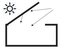
**Figure 2.24:** The sawtooth single clerestory scheme.
