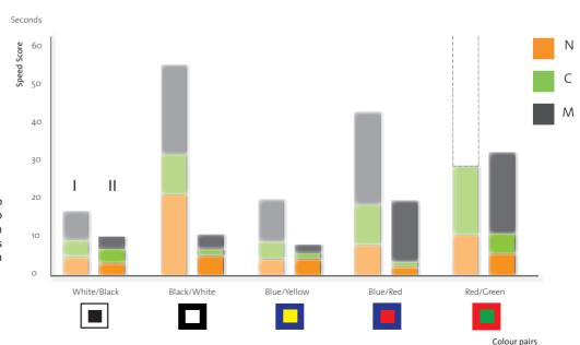
(3.7) The global Speed Score was split up into time employed by each category (N, C and M) to find book covers. For each colour pair, the column on the left (more opaque column) gives the results of the first lighting solution, while the column on the right represents the second lighting solution.
