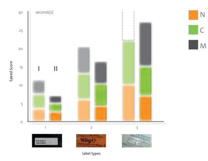
Chart 3.19 sums up the Speed Score showing the partial time of each subject category in the First (less opaque Column) and Second (more opaque Column) Solution. The vertical axis indicates the time (seconds), while the horizontal one the label types (1: high contrast, 2: medium contrast, 3: low contrast).
