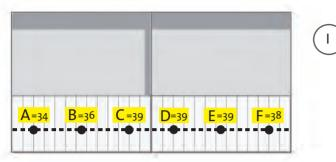
**Figure 3.30:** E values on the vertical grid at a distance of 8 cm from bookcase. I Artificial Lighting Solution.
