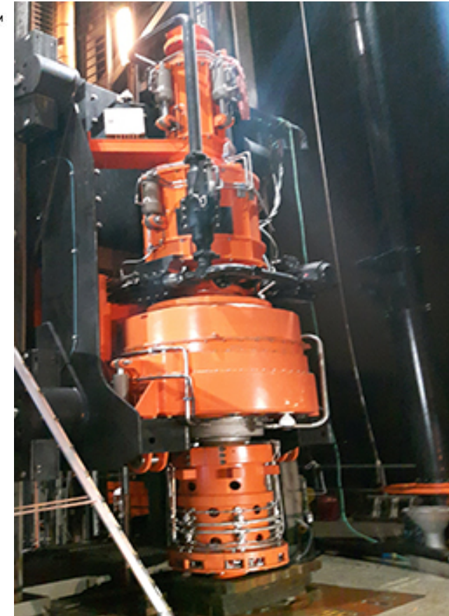
The Continuous Drilling & Circulation Unit (CDU) is offering the world's first continuous drilling operation. Photo: West Group.
