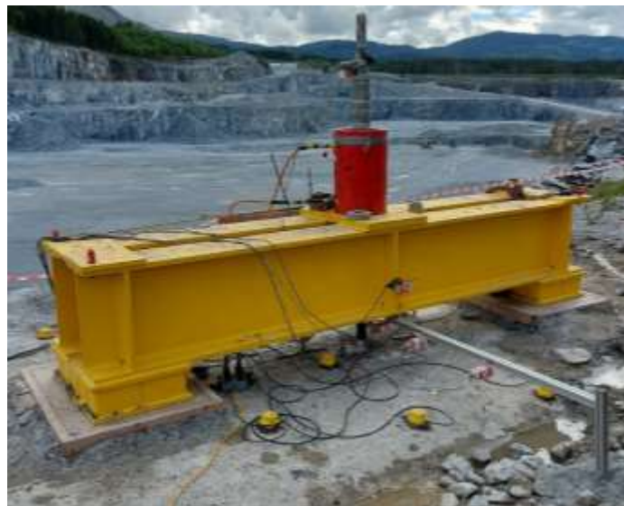
Figure 2. Test arrangement of anchor A1.5m. The steel beam is placed upon two concrete platforms with a hydraulic jack on top on the anchor. The LVDTs on the aluminium beam measured the surface heaving of the rock mass and the yellow geophones measured the microseismic activity during the test.
