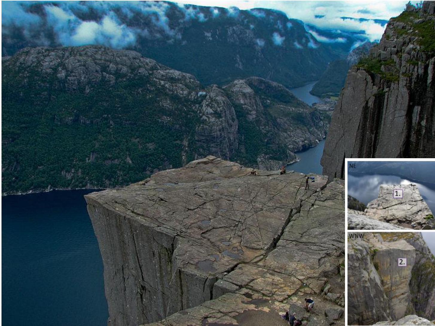
Figure 4.7: Five locations at Preikestolen were used to measure the point density of the point clouds. The point distance was measured for all the point clouds, using the point to point tool in CloudCompare. The locations were chosen to get a relatively even distribution of the measurements, with the main focus of the top plateau and lateral surfaces of Preikestolen.
