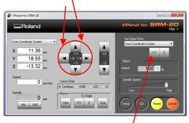
...after the XY alignment was done push X/Y button and confirm the action.
