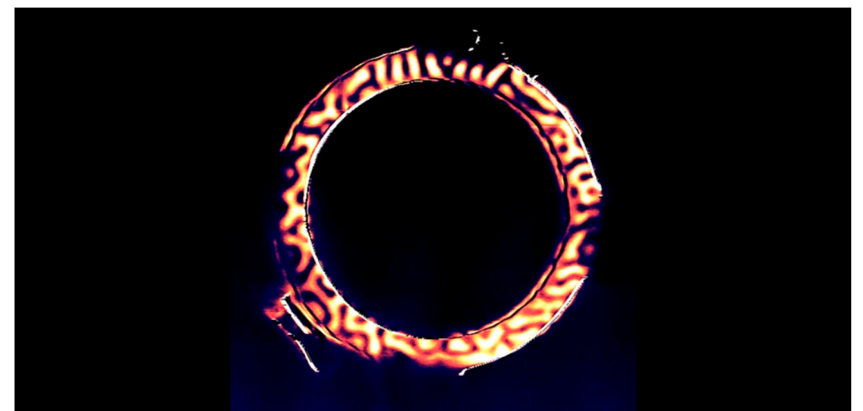
Magnetic domain pattern in a nano-structured ring. The contrast indicates the direction of the magnetization (dark: up; bright: down).
