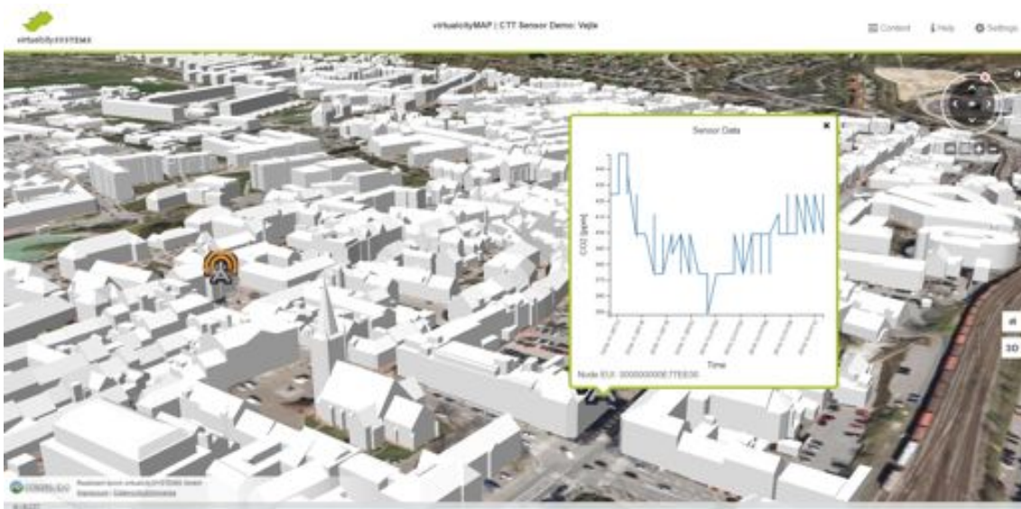
Figure 10 Visualizing the measurements of a sensor in a graph linked to a situated symbol in the 3D city map of Vejle.
