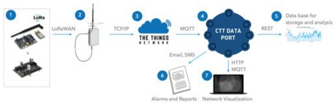
Figure 3 Network architecture and protocols
