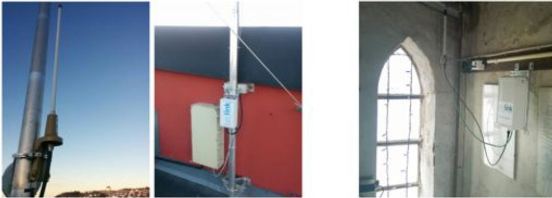
Figure 7 Deployment of LoRaWAN antenna gateway outdoors on the roof of the Student Society building in Trondheim (left) and elevated indoors in a clock tower in Vejle (right)
