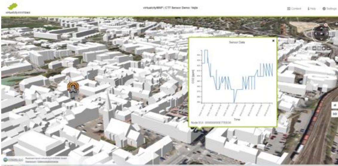
Figure 16 Visualizing the measurements of a sensor in a graph linked to a situated symbol in the 3D scene.
