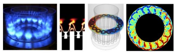
Annular instabilities and transient phenomena in gas turbine combustors
